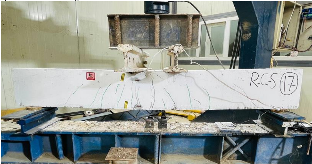
Figure 11. Beam RCS 17 after failure.
