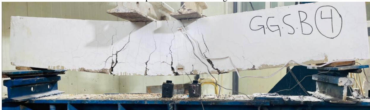
Figure 6. Beam GGSB4 after failure.
