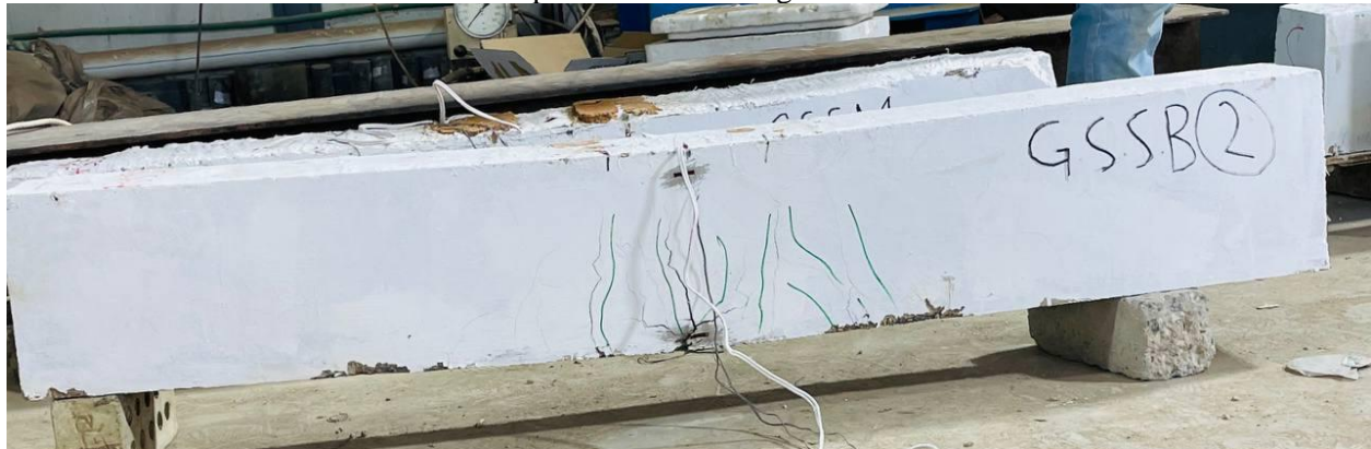
Figure 4. Beam GSSB2 after failure.
