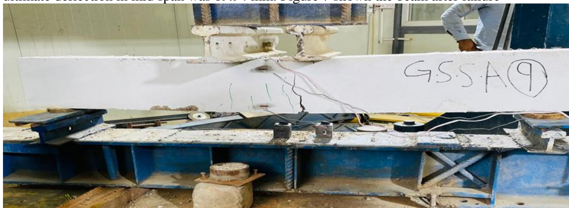
Figure 7. Beam GSSA9 after failure.
