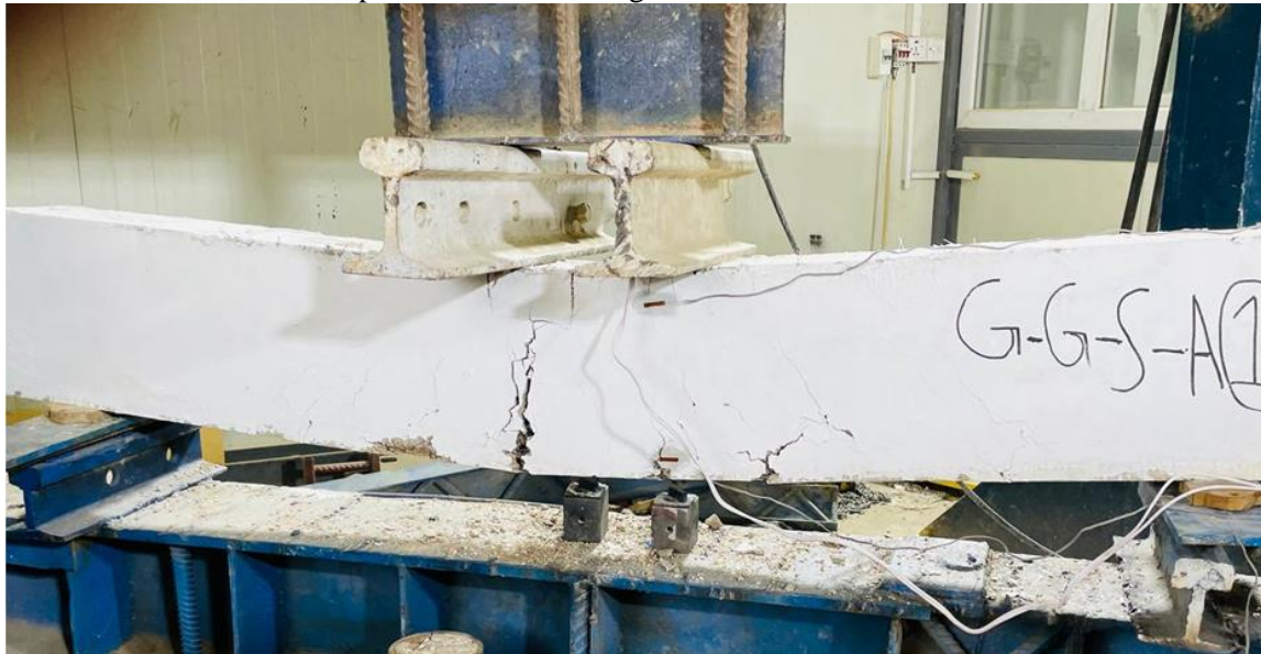
Figure 9. Beam GGSA11 after failure.
