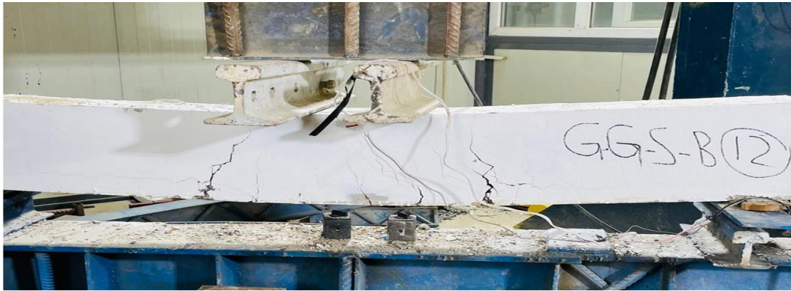
Figure 10. Beam GGSB12 after failure.
