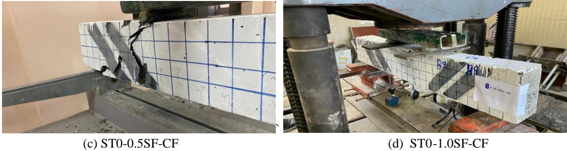
Fig. 10 Failure modes of the test beams as strengthened internally by SFRC or stirrups and with CFRP sheet.
